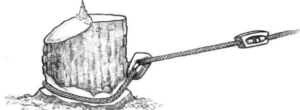
Figure 7-6 – Guyline Connectors – Poured Nubbins
