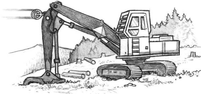
Figure 7-25 – Log Loader Anchor
